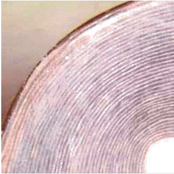
Fig. 1: Winding insulation. Note the different radii which cause the different bending of mica sheets (after [10])
