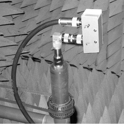
Fig. 7: The T-Resistive box in situ
